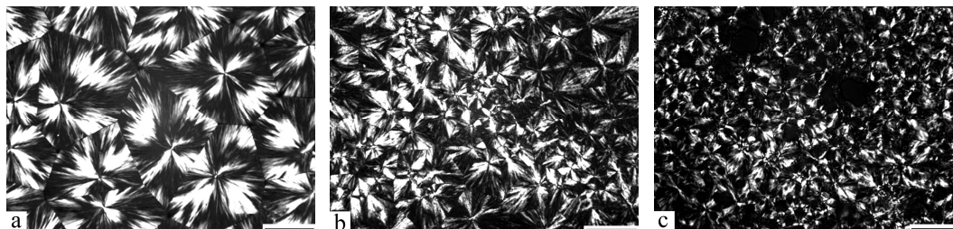
Fig. 8 Polarized optical micrographs of PLLA/PTMC blends with different PLLA/PTMC ratios: (a) 0/100, (b) 80/20 and (c) 60/40 (The scale bar is 10 \mu\text{m} .)
